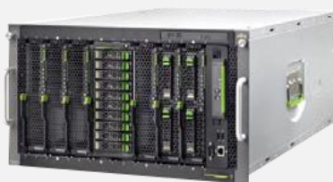
Fujitsu PRIMERGY BX400 Blade Enclosure
